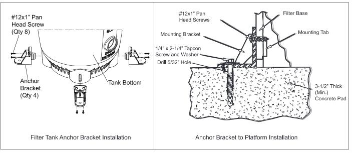
Figure 3. Anchor Filter to Equipment Pad
