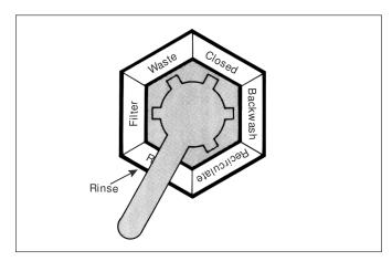
Figure 8. Diverter Valve Handle Positions
