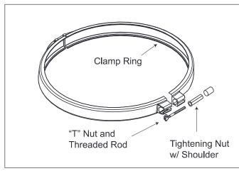
Figure 6. Filter Clamp Ring
