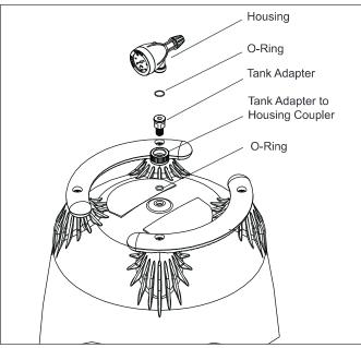
Figure 5. Pressure Gauge/Air Release Assembly
