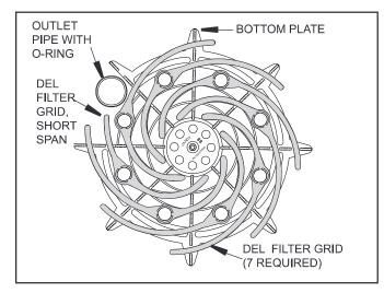
Figure 9. Filter Grid Arrangement
