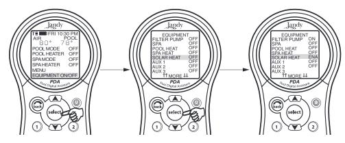
NOTE If no Solar Sensor is installed, EXTRAAUX will appear as a menu item.
