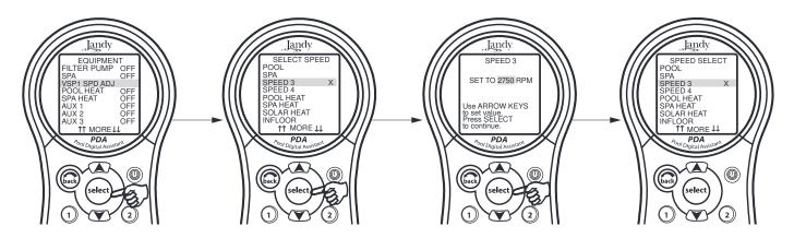
NOTE Speed adjustments from the EQUIPMENT ON/OFF screen are not permanent.
