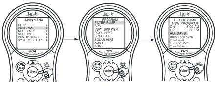
2. To run the variable speed pump at the SPEED3 setting from 8am to 1pm, highlight and select VSP SPD1 PGM, then highlight and select SPEED3, program it to turn on at 8am and off at 1pm.
