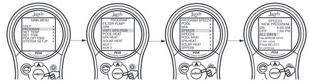
3. To run the variable speed pump at the SPEED4 setting from 1pm to 5pm, highlight and VSP SPD1 PGM, then highlight and select SPEED4, program it to turn on at 1pm and off at 5pm.
